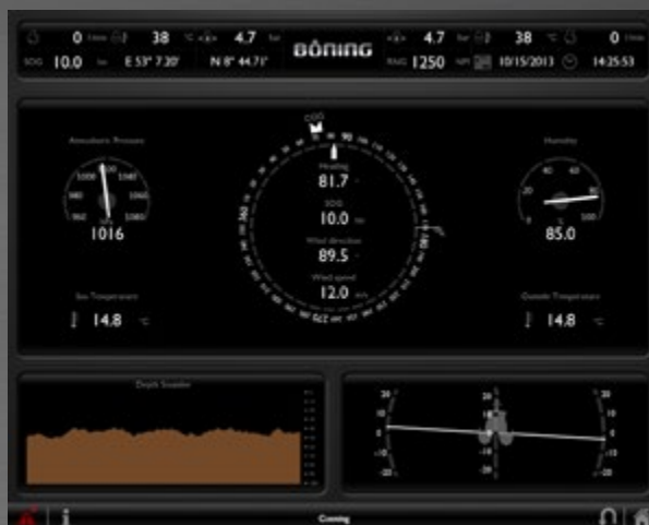
Conning page with navigational round instruments, such as air pressure, air temperature, humidity, COG, SOG, roll-pitch-yaw angle, and water depth.
