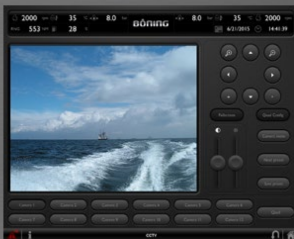
It is good to know what happens on board or in the close vicinity. Cameras in selected places monitor the corresponding areas. Comfortably controlled from the bridge, the display shows the desired images. Up to four fields can be viewed simultaneously on the display.
