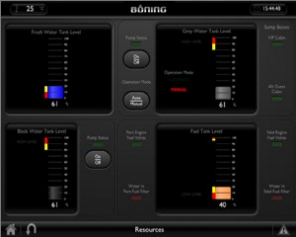
Fuel, water, oil, and other resources are carried along in tanks most of the time – as well as waste water and sewage. Bar graphs display the tanks' filling levels states. The pumps can also be controlled from this page.
