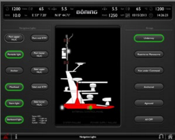
Navigation and signal lantern control and monitoring.
